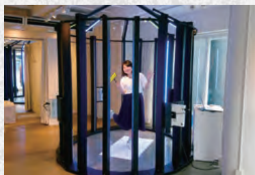
A 3D scanner installed at SR6
